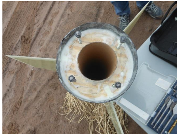
Figure 8 Motor mount system integrated into the rocket body (the thrust ring is not shown)
