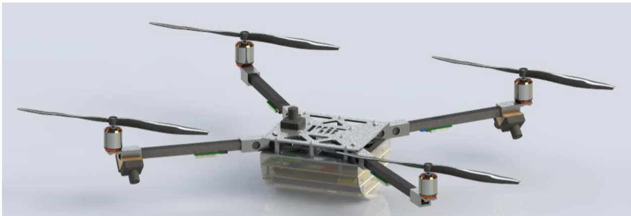
Figure 27 The Current Design of Quadrotor and Science Sensor Suite Configuration
