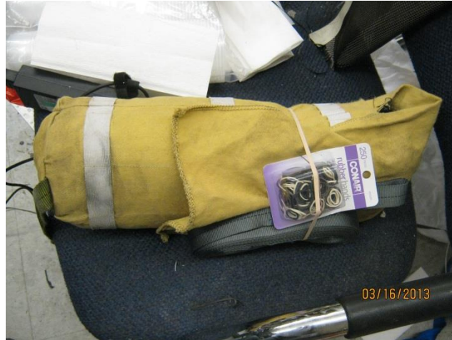
Figure 15 Parachute properly packed in deployment bag for full scale launch
