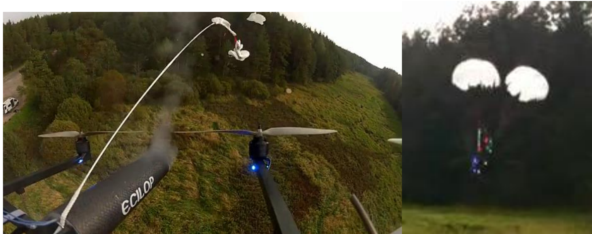
Figure 49 - The Ecilop deploying its parachute (left), and landing under parachutes (right). Images by Aleksey Zuitsevsky.
