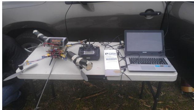
Figure 29 Ground station set-up (TV for video streaming downlink not shown)
